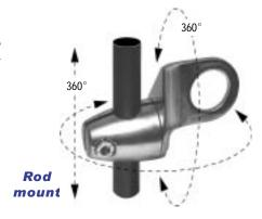
**How it works-** Two metal HalfKlamps attach and capture a Base, while they also secure a Bracket option to hold your sensor. Opposite the Bracket is a single adjustment fastener that is tighten to secures both the Bracket and HalfKlamp positions. The SoftNoze CUB™ puts you in ultimate control to position and securely lock sensors in place. A comprehensive selection of Base units and Brackets options allow you to harness the power of virtually any sensor and application!
