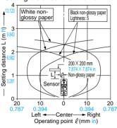
Correlation between material (200  $\times$  200 mm 7.874  $\times$  7.874 in) and sensing range
