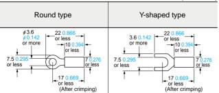
Note: Use crimp terminals with insulating sleeves. Recommended crimp terminal: Nominal size 1.25  $\times$  3.5 0.049  $\times$  0.138.
