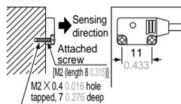
The tightening torque should be 0.2 N·m or less.
