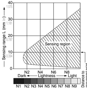
The sensing region is represented by oblique lines in the left figure. However, the sensitivity should be set with enough margin because of slight variation in products.
