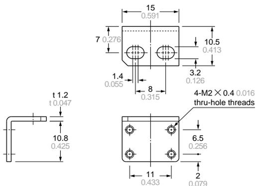
Material: Cold rolled carbon steel (SPCC)
