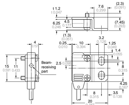
**DIMENSIONS (Unit: mm in)** The CAD data in the dimensions can be downloaded from the SUNX website: <http://www.sunx.co.jp/>
