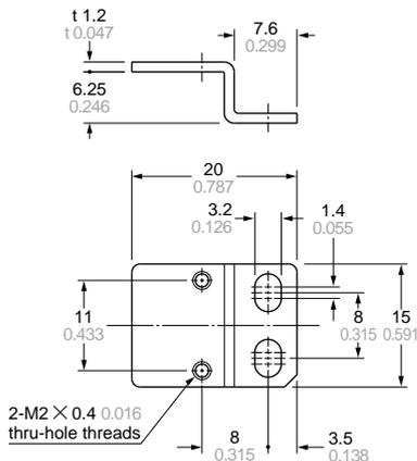
Material: Cold rolled carbon steel (SPCC)
