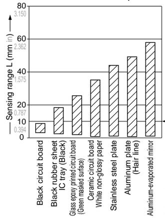
The bars in the graph indicate the sensing range for the respective material. However, there is a slight variation in the sensing range depending on the product. Further, if there is a reflective object (conveyor, etc.) in the background of the sensing object, since it affects the sensing, separate it by more than twice the sensing range shown in the left graph.
