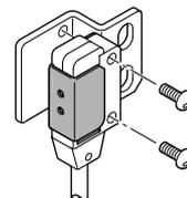
Tighten along with the sensor mounting bracket.
