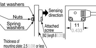
The tightening torque should be 0.2 N·m or less.
