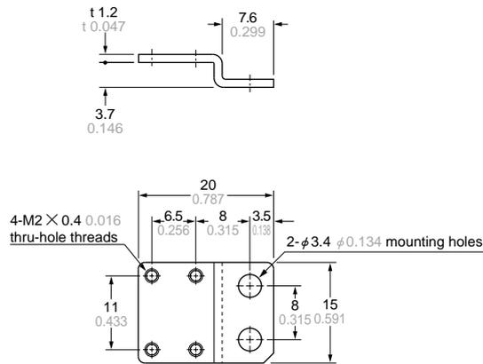
Material: Cold rolled carbon steel (SPCC)
