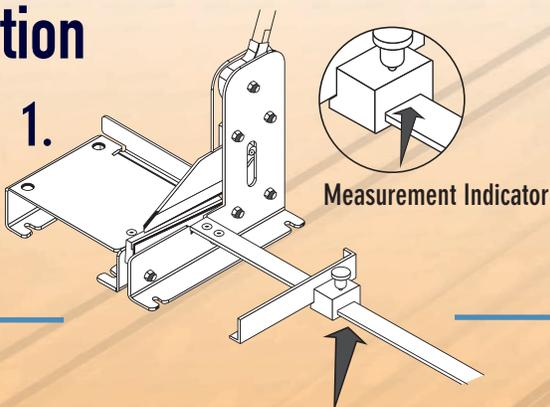
1. Adjust the desired length of the wiring duct by using the length stopper and lock position by screwing down the thumbscrew. Push down the blade guard with the wiring duct.
