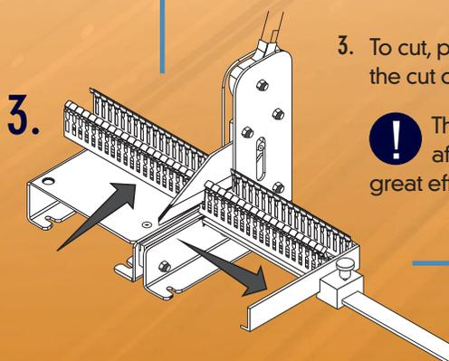
3. To cut, pull the level down. After the cutting, press the lever back up and carefully remove the cut duct parts. For this perhaps the length stopper has to be loosened.
