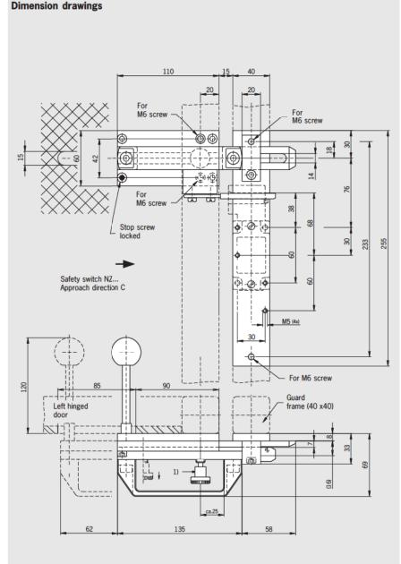
Bolt with detent mechanism:
