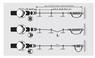
In order to achieve this, the rope pull switch has one center position and two switch-off positions. The switch is in center position during machine operation. If the safety rope is pulled or tears, the switch moves from the center position to one of the switch-off positions and the machine is stopped. Rope pull switches from EUCHNER have a sight window which allows the switch position to be seen.
