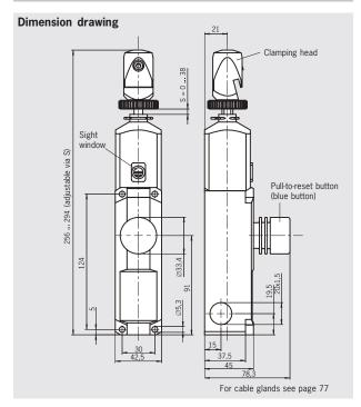
Cable entry M20 x 1.5 Turn-to-reset button for EMERGENCY-STOP, clamping head for tensioning rope
