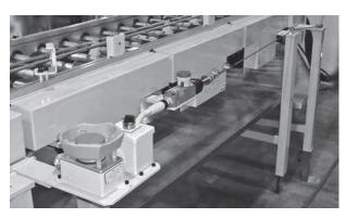
The advantage is that areas of an installation or machine can be shut down immediately from any point in the working area in the event of danger in cases where it would otherwise be necessary to install individual latched Emergency-Stop buttons at short distances apart.
