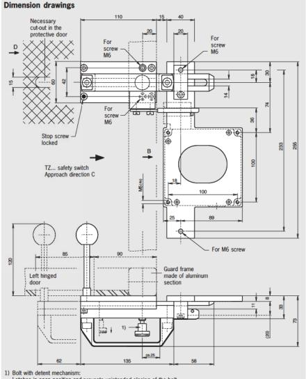
Latches in open position and prevents unintended closing of the bolt.
