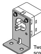
Two M3 (length 8 mm 0.315 in) screws with washers are attached.
