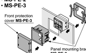
Panel mounting bracket **MS-PE-2**
